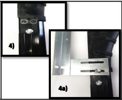
Before bolting on the flag bracket start with bolting together vertical track and plastic corner(4). Ones tight add the flag bracket on and set to approx. 70mm(4a)
