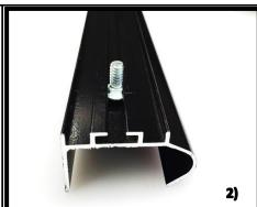
Start by sliding one bolt per every Jamb Bracket. By having a full length screw flute, jamb brackets can be moved to suit the available fixing points anywhere on the vertical track without having to drill new holes.
