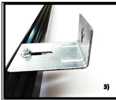
Set bottom jamb brackets approximately 100mm from the floor and for most 40mm thick doors set the track approximately 40mm from wall at the bottom and 70mm from wall at the flag bracket level. Adjust after second last panel is installed
