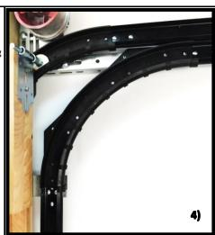
Low headroom set up shown is installed in 200mm headroom with vertical track cut to "ceiling height less 520mm". The main objective is to have the low headroom bracket flush or slightly higher than the panel. Bracket lower than the door may drive the door into the cable drum
